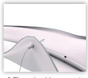
6.Thread cable support through eyelet.
